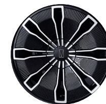
21" Turbojet type wheel with 40/265 R22 tire
