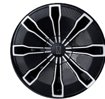
21" Turbojet type wheel with 40/265 R22 tire
