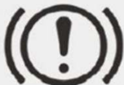
Fault warning lamp of brake system
